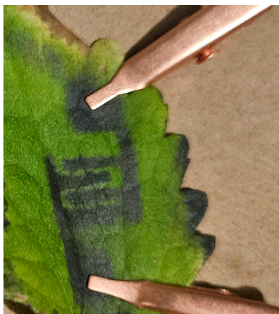
Figure A1. Connection of Wio Terminal device to leaf-deposited electrodes. Toothless (flat-jaw) crocodile clips were used to prevent mechanical injury to the leaf tissue.
